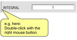
Offset calibration can be accessed by double-clicking with the right mouse button left of **INTEGRAL** in the **PARA** tab.
