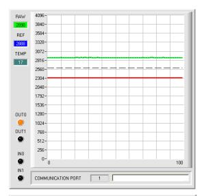
As long as the current measurement value **RAW** (green line) lies above the switching threshold (red line), the output **OUT0** has +24V (signal is OK). This is visualised by the **OUT0** LED.
