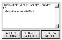
A click on the **GEN. HW INFO FILE** generates a file in which all the important sensor data are stored in encrypted form.
